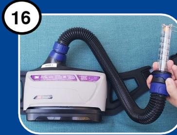
16 Insert the air flow indicator into the outlet of the breathing tube. With the air flow indicator in a vertical position, ensure the floating ball is at or above the minimum flow level.
