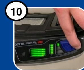
10 Turn the motor/blower ON. Let the unit run for 1 minute.
