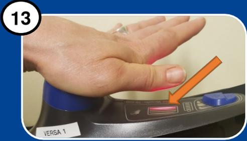
13 Perform a low flow alarm test by blocking air flow with your palm. The motor/blower unit should emit an audible alarm and show a flashing red light. In ~30 seconds If no alarm sounds, remove it from use and have it serviced. If the alarm sounds, proceed with these PAPR instructions.
