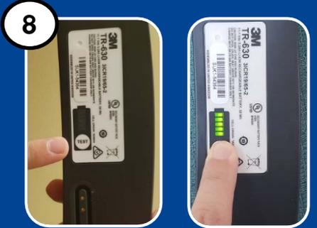
8 Press the TEST button on the bottom of the battery to confirm sufficient charge.
