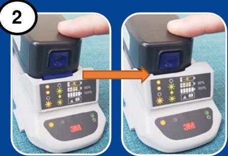
2 Charge the battery in the battery charger cradle prior to use. Ensure the battery clicks into place. The cradle will indicate the status of the battery charge.
