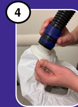
Prior to donning the headgear, ensure that the headgear is attached to the motor/blower with the breathing tube, the motor/blower is worn at the back and turned ON.
