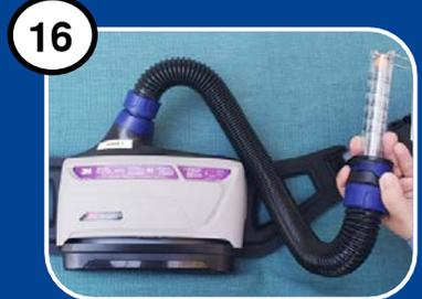
16 Insert the air flow indicator into the outlet of the breathing tube. With the air flow indicator in a vertical position, ensure the floating ball is at or above the minimum flow level.
