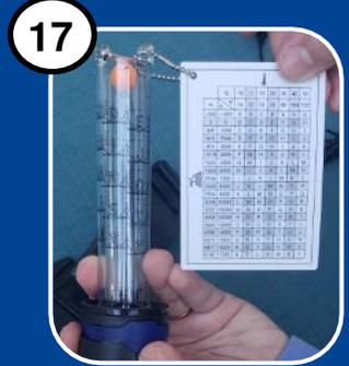
17 If not above the minimum level, re-inspect the breathing tube for blockage or damage. Replace the breathing tube if minimum air flow is not achieved, then re-check air flow. Turn motor/blower unit OFF to continue assembly.
