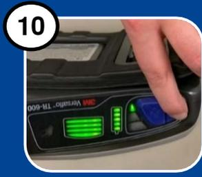
10 Turn the motor/blower ON. Let the unit run for 1 minute.
