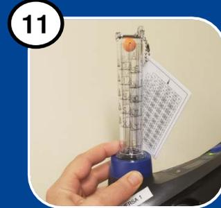
11 Insert the air flow indicator into the outlet on the motor/blower. With the air flow indicator in a vertical position, ensure the floating ball is at or above the minimum flow level for your zone on the attached chart.
