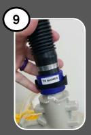
Attach the end of the breathing tube labeled "to blower" to the outlet on the blower by lining up the notches and pressing until a "click" is heard.
