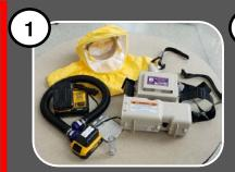
Inspect the PAPR components (motor/blower, breathing tube, battery, airflow indicator, belts/tabs, head gear, shoulder strap, foam block) to ensure that no parts are missing or damaged. Note the HEPA filter is **NOT** replaceable.
