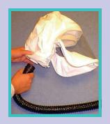
8. Connect the airflow tube to the plastic circle at the back of the head cover.
