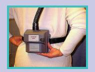
9. Place the PAPR (with airflow tube up) against your lower back and fasten the belt buckle.
