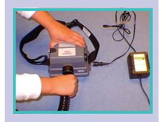
3. Check to ensure that the airflow tube is securely connected to the PAPR. Look for any signs of damage.
