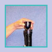
6. To check the airflow, place the "egg float" into the upright end of the airflow tube.
