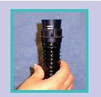
7. The lower band will rise above the edge of the airflow tube if the air supply is adequate.
