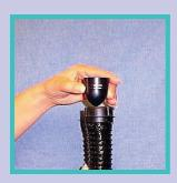
6. To check the airflow, place the "egg float" into the upright end of the airflow tube.
