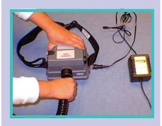
3. Check to ensure that the airflow tube is securely connected to the PAPR. Look for any signs of damage.
