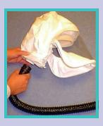
8. Connect the airflow tube to the plastic circle at the back of the head cover.
