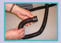
2. Inspect the airflow tube for cracks. Pay close attention to the end that connects to the head cover.
