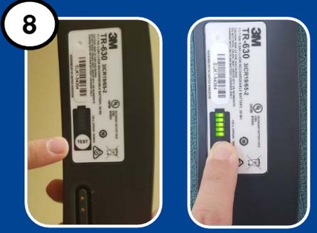
8 Press the TEST button on the bottom to confirm sufficient charge.
