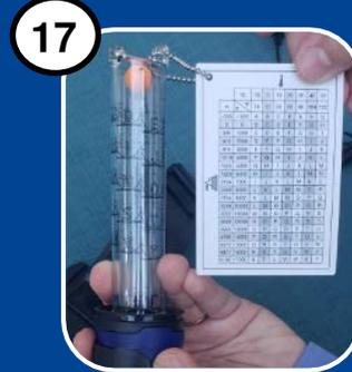
17 If not above the minimum level, re-inspect the breathing tube for blockage or damage. Replace the breathing tube if minimal air flow is not achievable. Turn motor/blower unit OFF to continue assembly.
