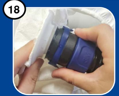
18 Attach the breathing tube to the hood. Push the end of the breathing tube into the air inlet of the hood while pinching the blue clip. You will hear a click. Gently pull to confirm the breathing tube is secure.
