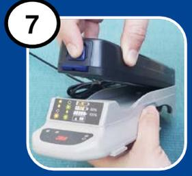
7 Remove the battery pack from the charger cradle by pressing on the blue button.
