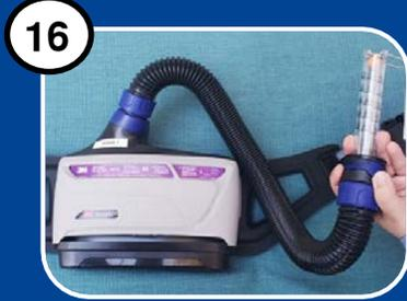
16 Insert the air flow indicator into the outlet of the breathing tube. With the air flow indicator in a vertical position, ensure the floating ball is at or above the minimum flow level.
