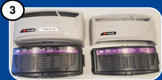
3 If using a filter cover, the size of the filter cover must match the size of the filter/cartridge provided to you for your specific job hazards. Chemical/HEPA cartridge shown at left (**BLACK/PURPLE** label) and HEPA filter shown at right (**PURPLE** label).
