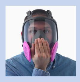
Place the palm of your hand over the opening in the exhalation valve cover and exhale gently. If facepiece bulges slightly and no air leaks are detected between the face and the facepiece, a proper seal has been obtained. If faceseal air leakage is detected, reposition the respirator on your face and/or readjust the tension of the straps to eliminate leakage and recheck seal. If you cannot achieve a proper seal, DO NOT enter the contaminated area. See your supervisor.
