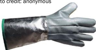
This extreme heat-protection glove with a sleeve, is rated for temperatures up to 900 °C for 20 seconds. It should be used in muffle furnace processes that are not to exceed 800 °C.
