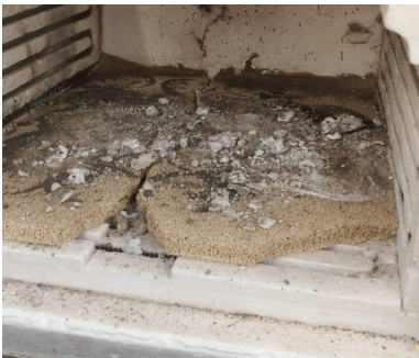
Debris from meltdown and combustion of plastic material placed in a muffle furnace with glass objects. Photo credit: anonymous
