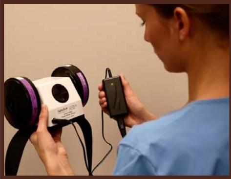
The light on the battery charger is green when the PAPR is fully charged.
