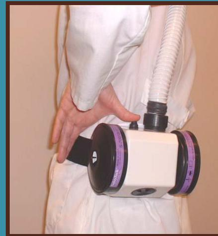
Slide the PAPR over on it's belt and turn it on by pressing the button **HARD** until you hear a click. The PAPR will beep four times to verify airflow, then the head cover will inflate.
