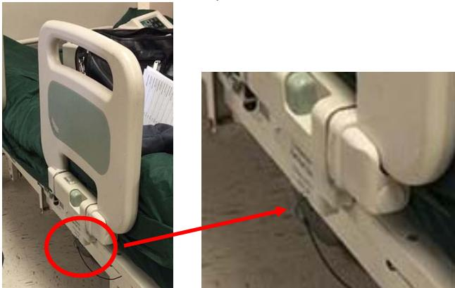
2. Pull up on bed rail to remove from bed.
