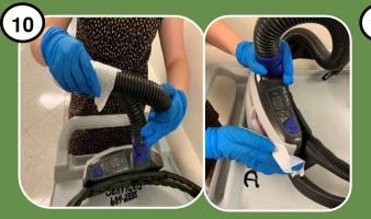
Use disinfectant wipe(s) to thoroughly disinfect the outside of the motor/blower and breathing tube.
