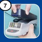
Remove the battery pack from the charger cradle by pressing on the blue button.
