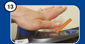
Perform a low flow alarm test by blocking air flow with your palm. The motor/blower unit should emit an audible alarm and show a flashing red light. In ~30 seconds If no alarm sounds, remove it from use and have it serviced. If the alarm sounds, proceed with these PAPR instructions.
