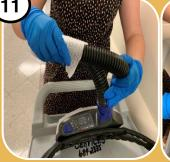
Use disinfectant wipe(s) to thoroughly disinfect the outside of the motor/blower and breathing tube.
