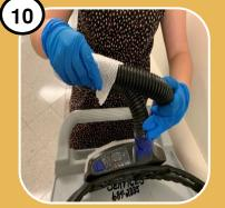
Use disinfectant wipe(s) to thoroughly disinfect the outside of the motor/blower and breathing tube.
