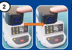
Charge the battery in the battery charger cradle prior to use. Ensure the battery clicks into place. The cradle will indicate the status of the battery charge.
