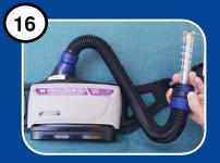
Insert the air flow indicator into the outlet of the breathing tube. With the air flow indicator in a vertical position, ensure the floating ball is at or above the minimum flow level.
