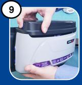
Attach the battery pack into the bottom of the motor/blower. A distinct click will be heard. Gently pull the battery to ensure it is firmly attached.
