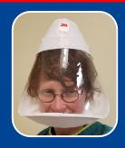
A properly fitting hood will be comfortable to wear and protect the user as intended. In these photos, the small circumference of the head suspension does not allow the comfort pad to be worn at the forehead. Additionally, the visor is too close to the face.
