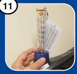
Insert the air flow indicator into the outlet on the motor/blower. With the air flow indicator in a vertical position, ensure the floating ball is at or above the minimum flow level for your zone on the attached chart.
