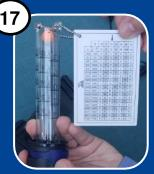
If not above the minimum level, re-inspect the breathing tube for blockage or damage. Replace the breathing tube if minimal air flow is not achievable. Turn motor/blower unit OFF to continue assembly.
