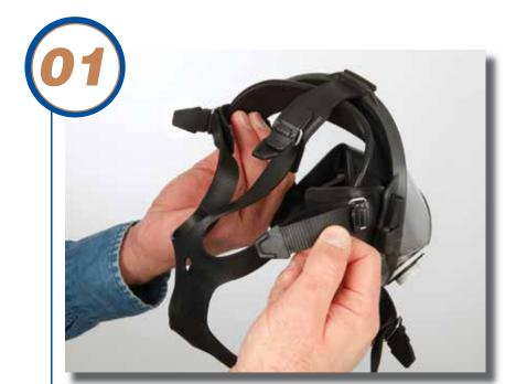
Check the facepiece seal & headstraps (or headnet suspension) to make sure they are in good condition, without any holes or tears. Check the cartridge connectors to make sure they are not cracked and are fully inserted into the mask.
