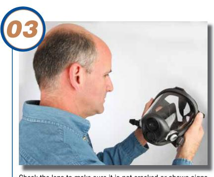
Check the lens to make sure it is not cracked or shows signs of crazing.
