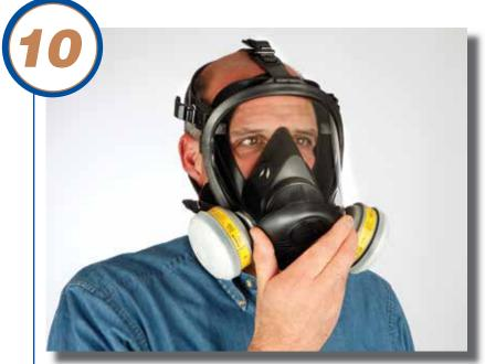
Start by placing the top of the nose cup over the bridge of your nose. Bring the bottom of the nose cup to your chin, centering the mask on your face. Holding on to the mask nozzle, press towards your face until you achieve full face-to-seal contact.
