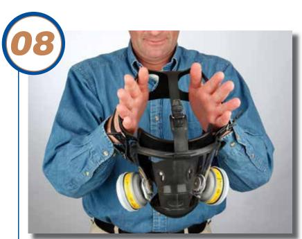
Grasp the headstrap harness, with your thumbs positioned through the straps. Spread the straps outward.
